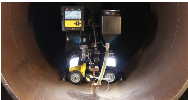
Versotrac with 3 wheels inside a pipe and with optional LED lamp kit
